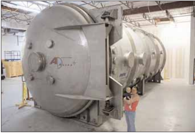
Figure 5. Ad Astra Rocket Co.'s new 35-foot-long, 15-foot-diameter vacuum chamber
