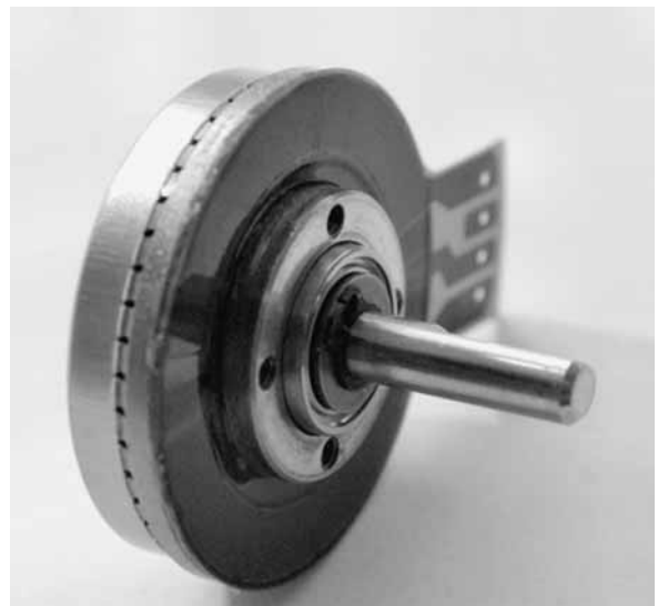
Figure 1. Piezo Systems ultrasonic motor (Shinsei USR30)
